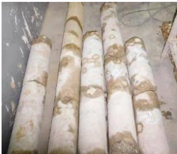
Figure 5. Concrete cantilever wall samples
