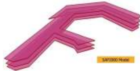
Figure 12. SAP2000 3D model for the slab bands
