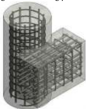
Figure 2. Rebar intersection representation
