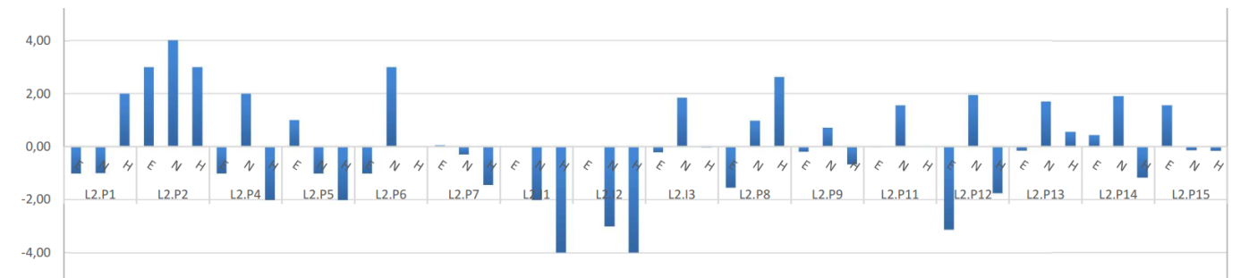
Deformation on Peripheral Retaining Walls – Lot 2 (mm)
