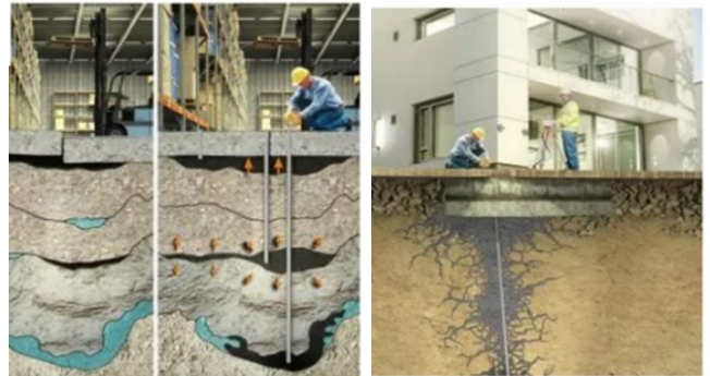
Injection system - Uretek Floor Lift ( https://www.uretek.pt )
