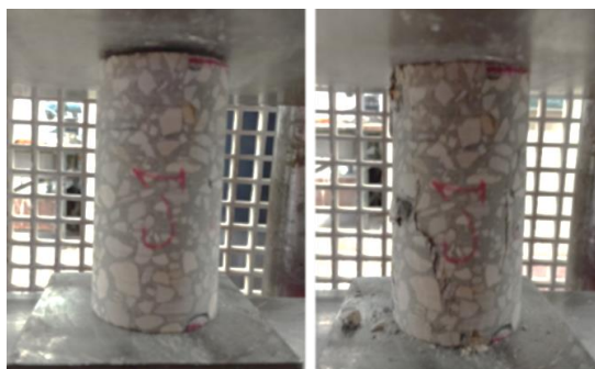
Figure 6. Uniaxial compression-strength testing – UCS.
