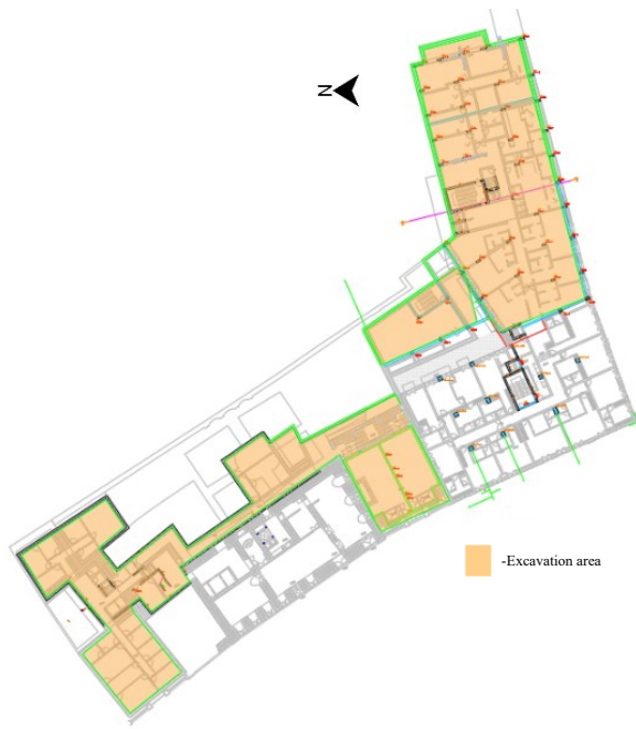
Figure 2 - Areas to be excavated under the existing structure.
