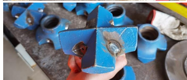
Figure 4. View of the micropiles hollow bars and bits.
